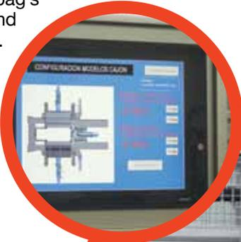
The MAC 100 is a flexible system that adapts to different size bags automatically. The robot adjusts the machine format (from the smallest to largest bags). Various programmed sizes can be stored and immediately recalled through the touch screen that automatically re-calibrates the system for fast changeover.
