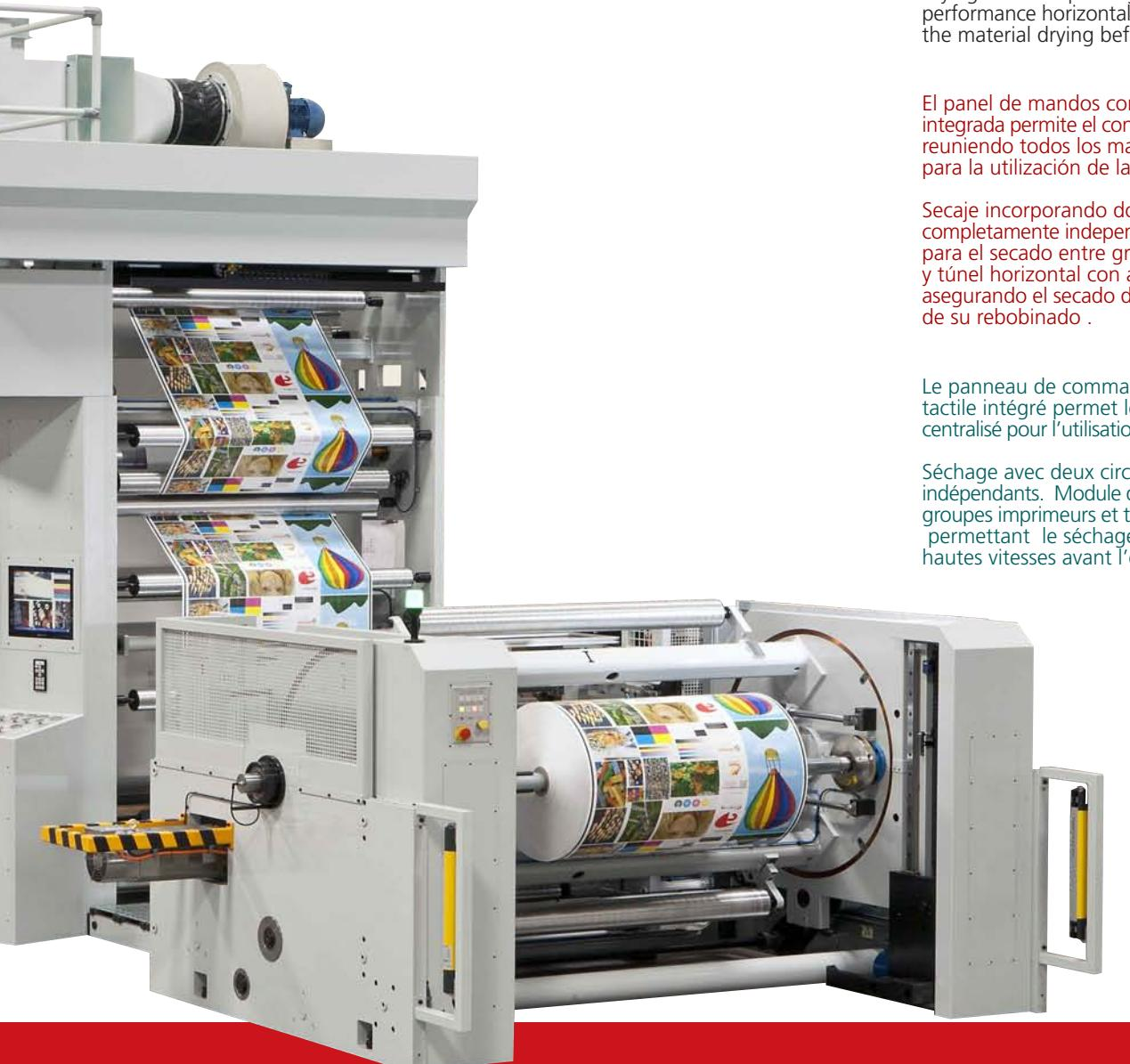
MIZARFLEX series offer unwinders and rewinders of totally automatic change or double-station for semi-automatic change. Diameters to 1.200 mm.
