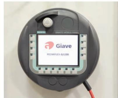
The integrated control panel allows the centralized control by a touch screen, including all the necessary control for the machine use.
