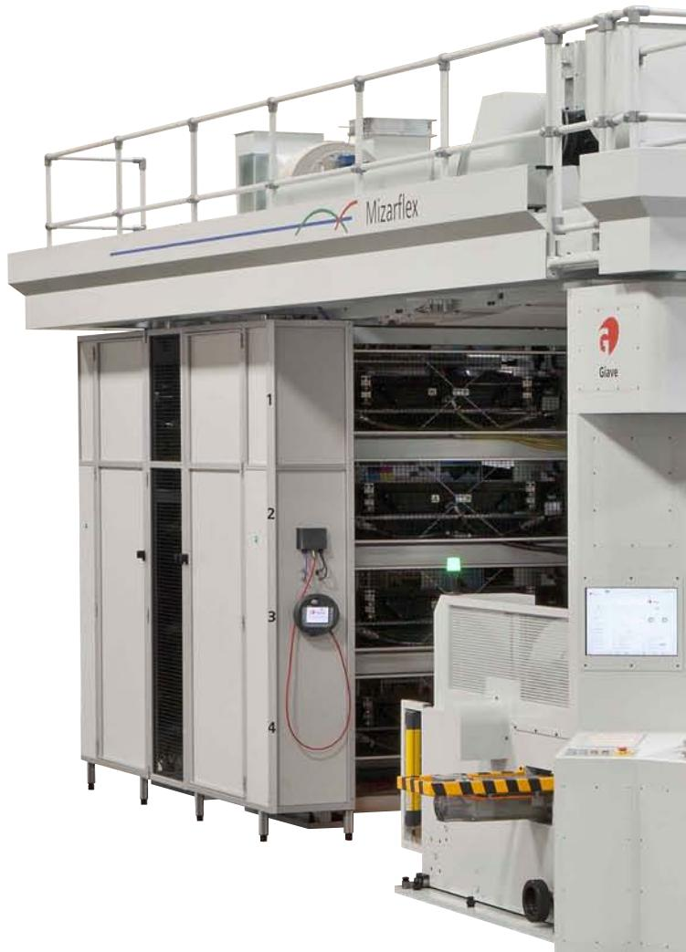
In MIZARFLEX series, each backpressure roller, plate cylinders, anilox and pressure adjustments are operated by independent servomotors.
